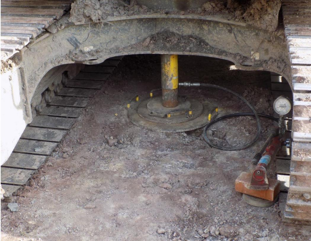
Following the bearing pressure tests work was carried out to remove unsuitable material from the base of the slope to locate bed rock.
